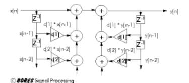
The filter diagram can show what hardware elements will be required when implementing the filter:
