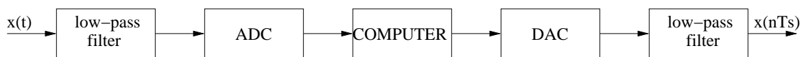
Figure 2: Low-pass filters in a digital audio system ensure that signals are bandlimited.
