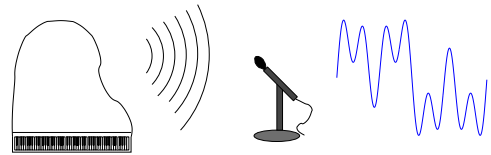
Figure 1: The electrical signal used to represent the pressure variations of a sound wave is an analog signal.
