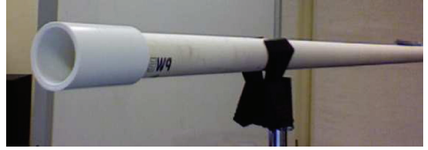
FIGURE 10: Instrument I3 is created to verify results that account for the junction created by appending a second tube object to the original measurement tube. It has a cylindrical open-end reflection which may, like that of instrument I2, be validated through comparison with theoretical expectation.
