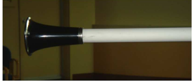
Figure 5. Adapted measurement system, showing a clarinet bell appended to the measurement tube, allowing for measurement of the clarinet bell reflection filter.
