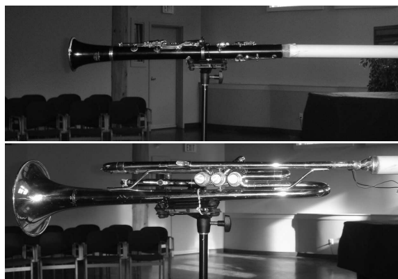
Figure 4. The clarinet and trumpet reflection functions are measured by appending them to the calibration cylinder.
