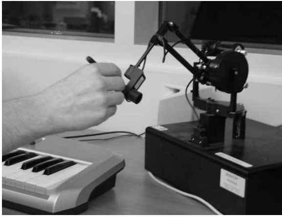
Fig. 3. A user controlling the virtual reed model using a Phantom and a MIDI keyboard.
