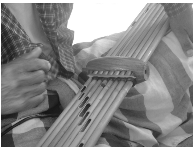
Figure 1: Mr. Khene, a khaen maker from Roi Et, Northeast Thailand, displays the tuning vents in the pipes.
