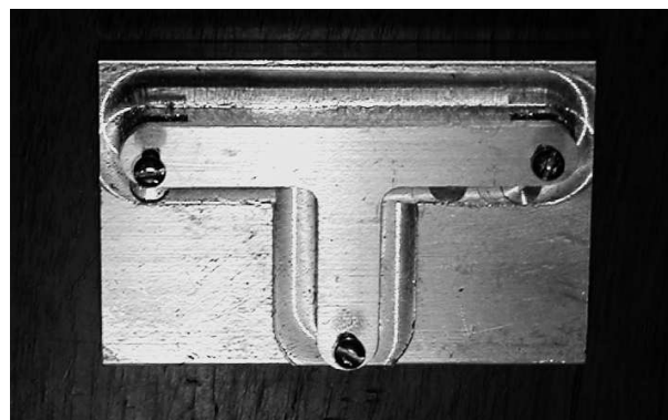
Figure 4: Fixturing the T-part for CNC machining
