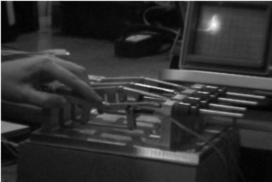
Figure 3.8: The signal (as viewed on the background oscilloscope) after passing through the signal conditioning circuit in Figure 3.7 representing the energy generated by the downbuckling of a rib.
