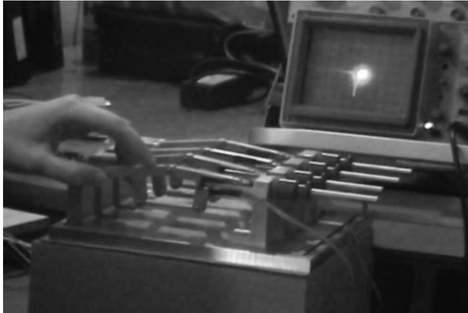
Figure 3.9: The signal (as viewed on the background oscilloscope) after passing through the signal conditioning circuit in Figure 3.7 representing the energy generated by the upbuckling of a rib.
