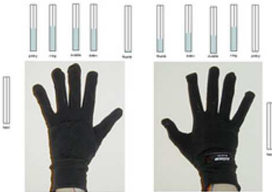
Figure 2.12: A Max (MSP) patch is used to demonstrate the sensitivity and resolution of the sensors. Each finger and heel of the glove is mapped to a level meter, and gives visual feedback to the amount of pressure being applied.
