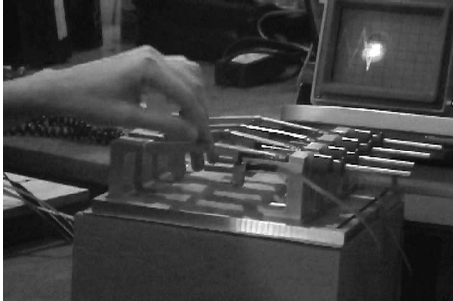
Figure 3.11: A sequence of up and down pulses can be seen on the oscilloscope (in the background) during normal playing.
