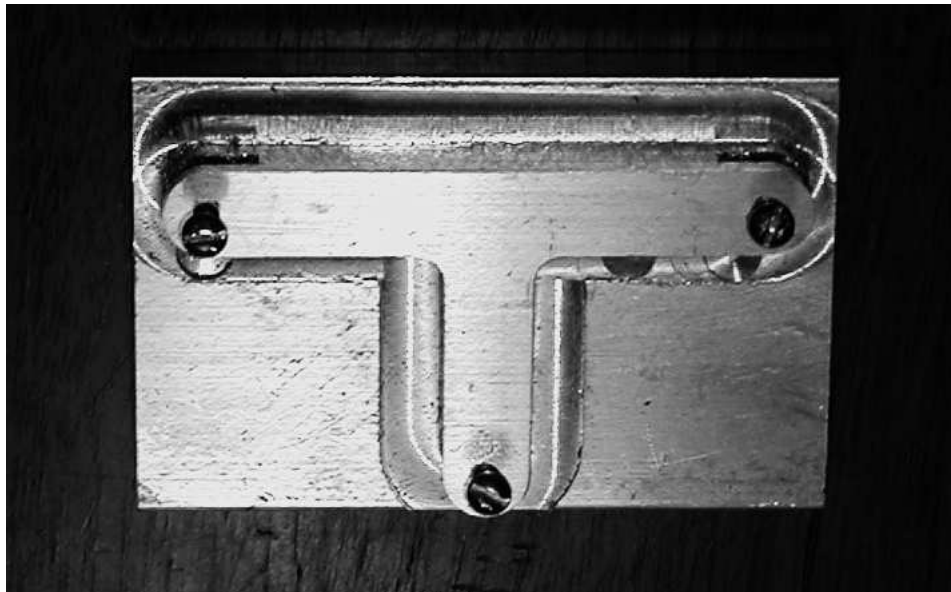
Figure A.1: Fixturing the T-part for CNC machining.
